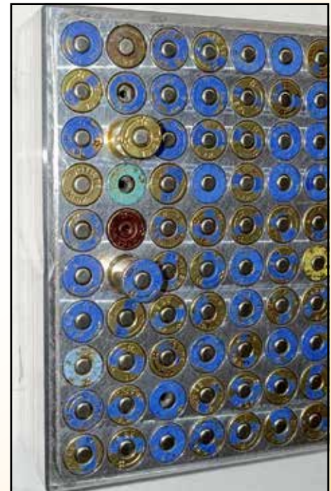
IN THIS 100 ROUND DEMONSTRATION YOU CAN SEE HOW WE CATCH A LOT OF BAD ROUNDS ON THE OUTSIDE. THEN WHEN YOU EMPTY, THE STUCK BAD ROUNDS WILL ANNOUNCE THEMSELVES.
