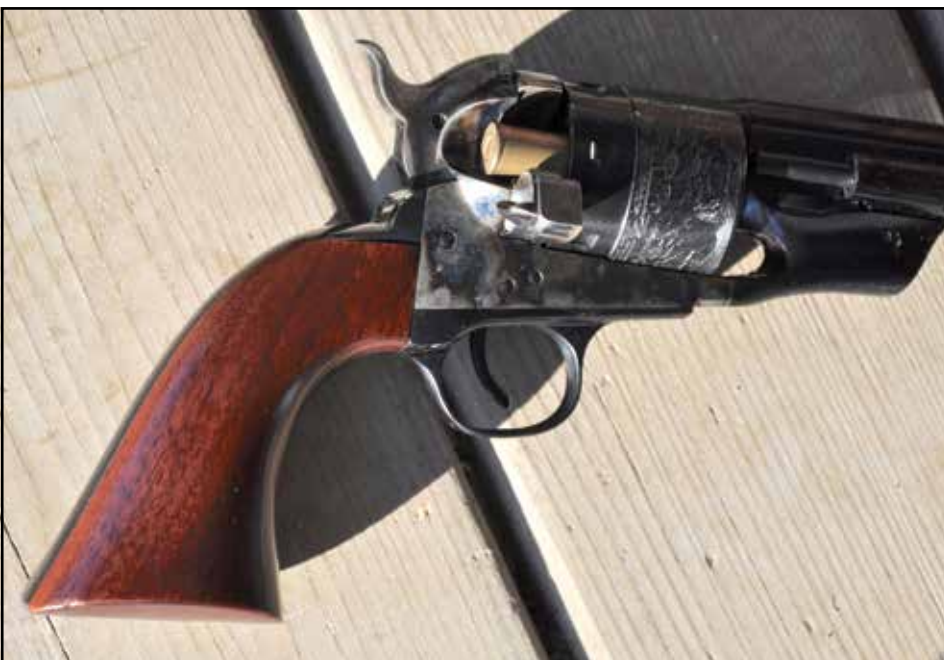
LOADING GATE OF THE TYPE II RICHARDS IS SIMILAR TO THAT OF THE LATER 1873 COLT.
