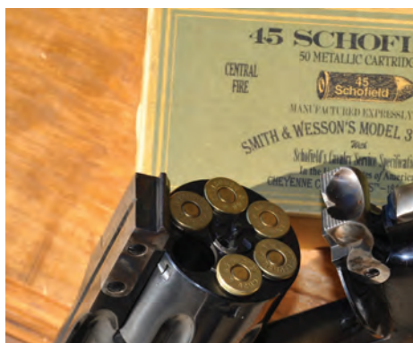
THE SCHOFIELD'S "TOP BREAK" ACTION PARTIALLY OPEN.
