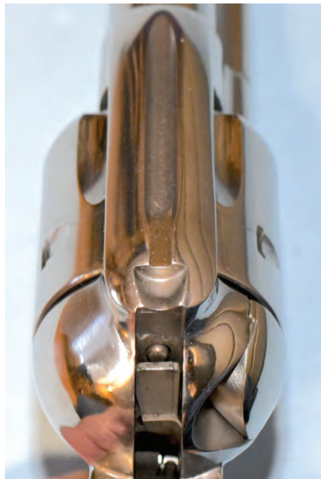
TRANSFER BAR IN THE "SAFETY" POSITION. HAMMER CANNOT STRIKE THE FIRING PIN.
