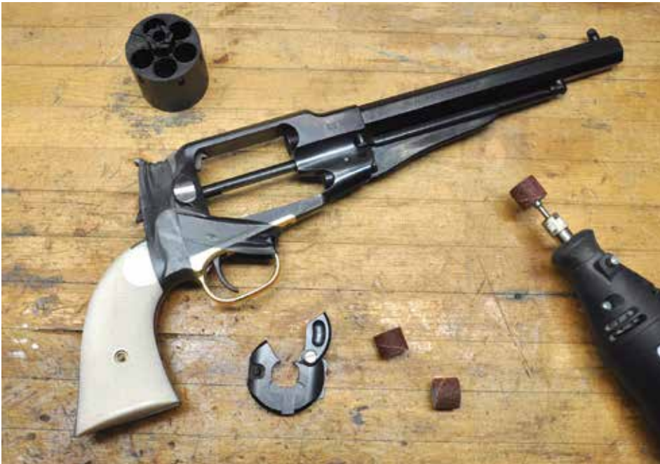
PIETTA 1858 DISASSEMBLED AND CARTRIDGE LOADING CHANNEL STARTED.
