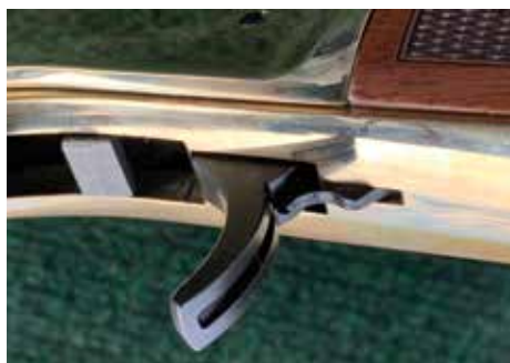
TRIGGER WITH TRANSFER BAR SAFETY. TRIGGER IS BLOCKED UNTIL LEVER IS COMPLETELY CLOSED.
