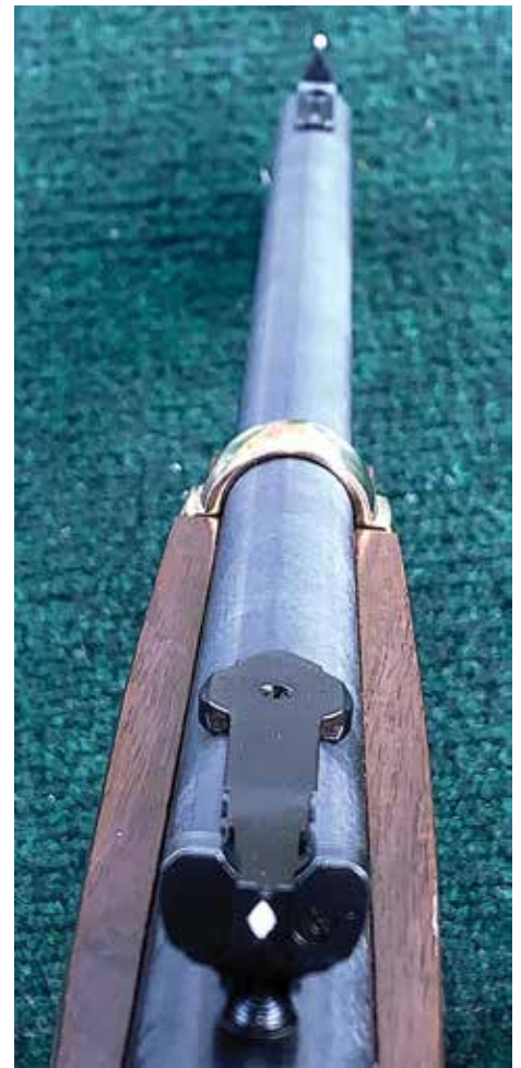
REAR SIGHT IS THE MARBLES SEMI-BUCKHORN. FRONT IS RAMP WITH IVORY BEAD.
