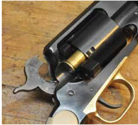
FINISHED LOADING CHANNEL WITH COLD BLUE.
