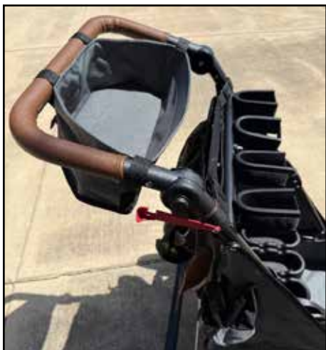
THE ADJUSTABLE HANDLE HAS A WELL DONE LEATHERETTE COVER. IT ADJUSTS FROM VERTICAL TO PAST 90 DEGREES. THE LOADING POCKET IS DEEPER THAN BEFORE.
