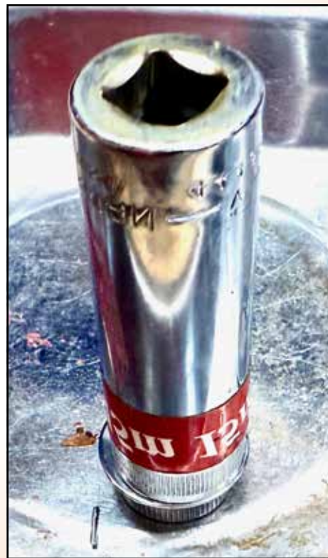
A DEEP SOCKET THAT FITS ACTS AS A WEIGHT TO KEEP THE WASHER TIGHTLY PACKED.
