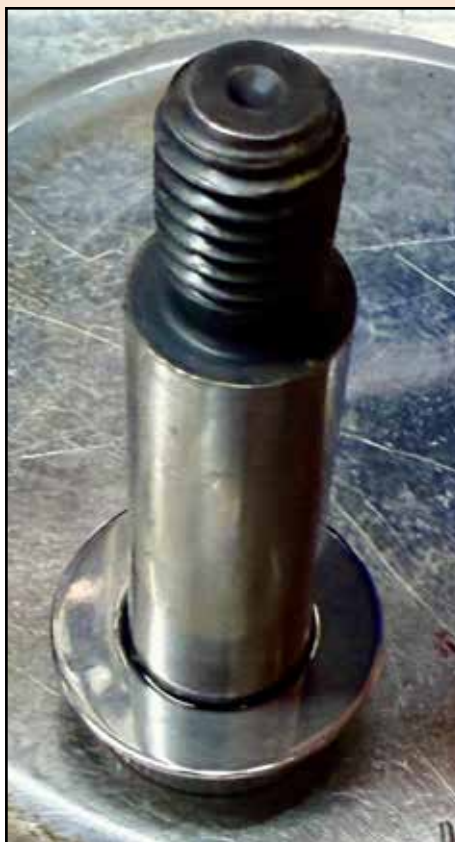
THE SHELL PLATE BOLT IS UPSIDE DOWN, CLEANED AND POLISHED. FOUR DROPS OF LOCTITE 609 ARE ON THE UNDERSIDE OF THE BOLT HEAD. THE THRUST WASHER, CLEANED WITH ALCOHOL, IS SLID DOWN THE BOLT TO SIT ON THE BOTTOM OF THE BOLT HEAD AND TURNED 90 DEGREES, SPREADING THE LOCTITE EVENLY, THEN LEAVE IT ALONE FOR SEVERAL HOURS, MAYBE OVERNIGHT.
