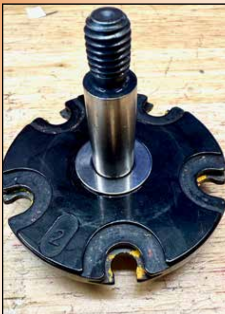
THE BOTTOM THRUST WASHER IS ATTACHED TO THE SHELL PLATE WITH 609.
