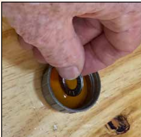
THE NEEDLE BEARING IS WET WITH A SYNTHETIC OIL SUCH AS MOBIL 1.
