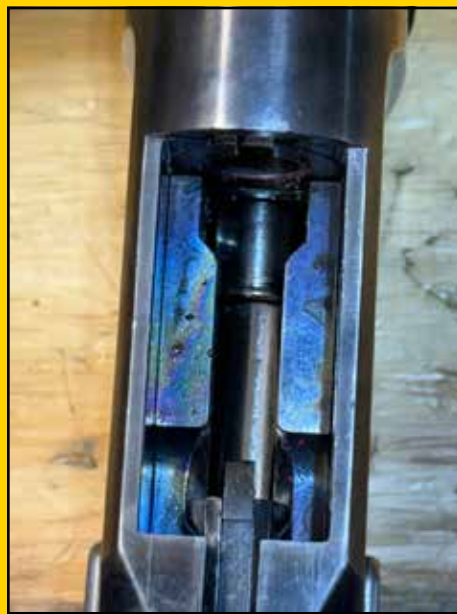
ROUND JAMMED, WILL NOT GO INTO CHAMBER, COULD BE SPLIT CASE ALLOWING THE BULLET TO RETRACT INTO THE CASE, TOO SHORT A BULLET, OR JUST NOT YOUR DAY.
