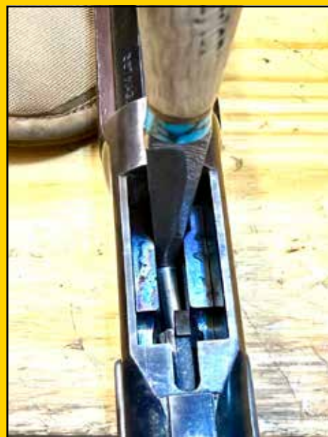
SCREWKNIFE PUSHED DOWN BETWEEN ROUNDS, ALLOWING THE CARRIER TO PICK UP THE REAR ROUND AND LINE UP TO EXTRACT IT OUT THE LOADING GATE.
