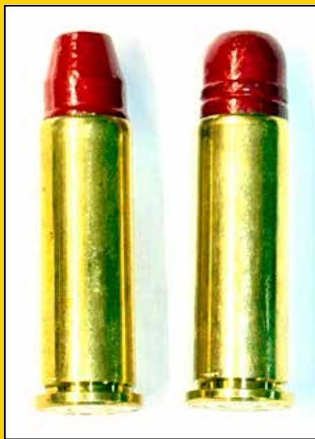
105-GRAIN COATED TRUNCATED CONE ROUND LOADED TO 1.50" OAL AND 158-GRAIN COATED ROUND NOSE FLAT POINT LOADED TO 1.49" OAL. THE LOADING DIES DO NOT HAVE TO BE READJUSTED BETWEEN THE DIFFERENT BULLETS.
