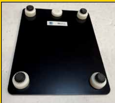
BOTTOM VIEW OF THE SCALE LEVELING PLATFORM SHOWING LEVELING FEET.
